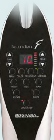
programmable presets and manual control with 7 scalp temperature levels
