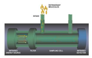
The filtered infrared energy passes through the sampling cell, striking the infrared detector. D-Tek CO2 is ready to sense any CO2.
