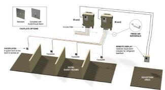
**RD-em** based Refrigerant Leak detection system for Hotel/multi-room application. RD-em can also be sold as a standalone device
