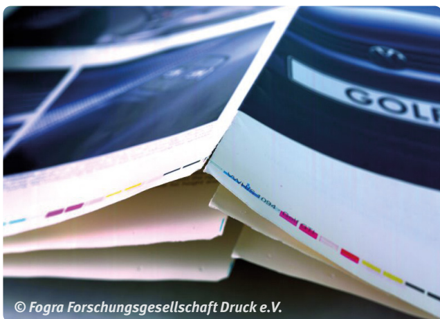
Fig. 11: Breaking in the fold in lightweight papers
