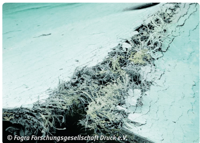
Fig. 12: Broken folds can cause press stoppages
