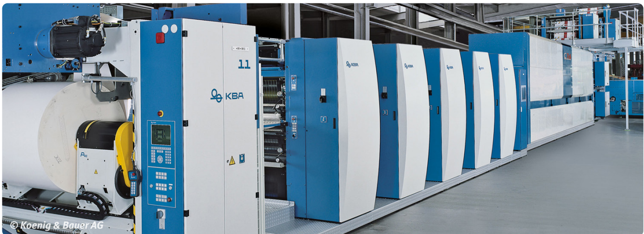
Fig. 7: Web offset printing press with drying oven
