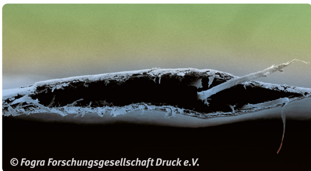
Fig. 9: Tearing in the internal structure of the paper
