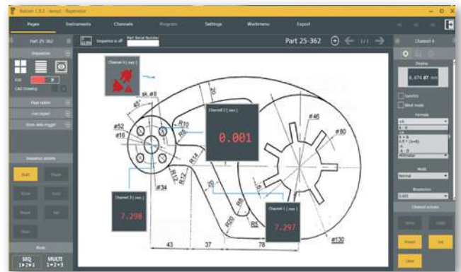
Display of the measurement of a multi-dimensional part with drawing of the part in the background
