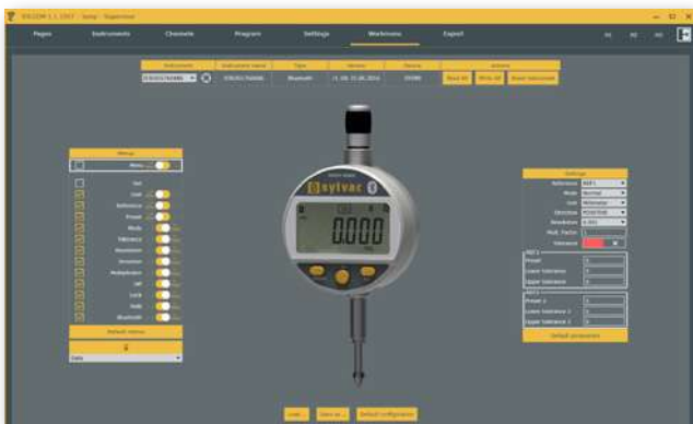
Work menu: program the menu of your instrument directly via Sylcom
