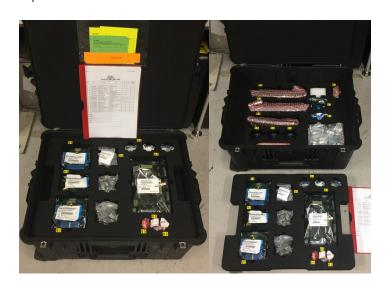
The result was a series of kits made from secure, robust and portable cases which protected its contents from vibration and impact - CP Cases recommended Injected Moulded Cases with wheels and foam engineered pockets and pouches. Each part has a designated slot and each time it was consumed the engineer simply ordered a replacement. An index list per kit tracked usage.
