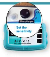
Control box Attaches to bed using velcro or protective rubber case
