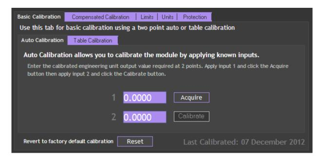
The automatic calibration requires that you apply two known (ascending) weight in sequence. Just enter the required engineering unit value for the two weights in the fields marked 1 and 2.
