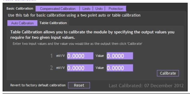
This option lets you calibrate direct from the loadcell manufacturers certificate without having to apply weights to the input.
