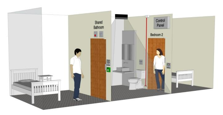
There are minimum standards for disabled toilets regarding the size of entrance and the space needed for manoeuvring a wheelchair through 180 degrees. There is also a recommended minimum of 700mm to allow a wheelchair user to slide from chair to toilet. The exact design and layout will depend upon local circumstances and any system should be considered with the architect at the design stage.
