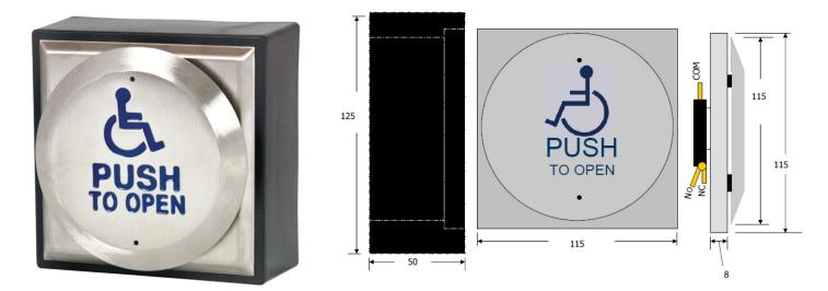
Surface mount stainless steel plate 100mm Round Switch with Disabled Logo and text engraved 'PUSH TO OPEN' SPCO contacts rated at 2A 48vdc or 15A 250vac
