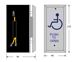
Surface mount stainless steel plate narrow style engraved with disabled logo and "PUSH TO OPEN" SPCO contacts rated at 2A 48vdc or 15A 250vac
