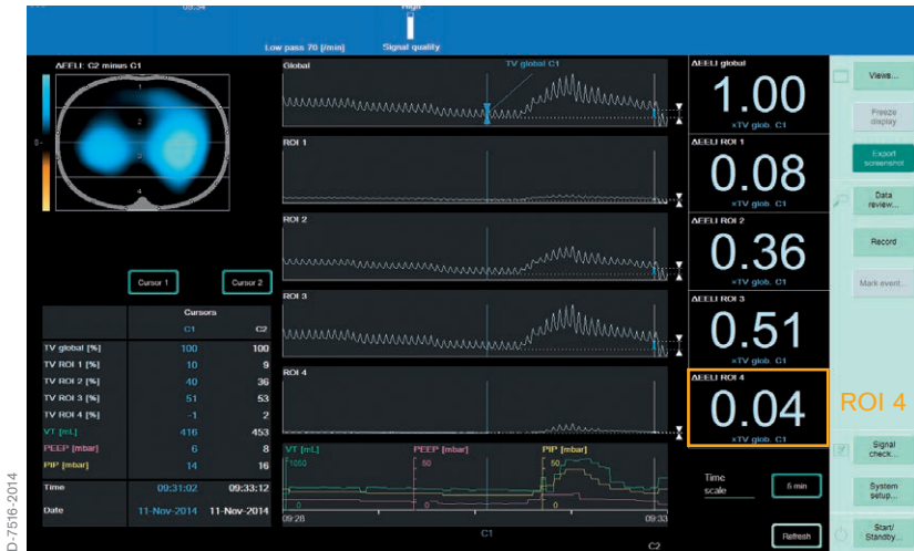
Fig. 35: Trended distribution of \Delta EELI , where the status before and after a recruitment manoeuvre is compared. The differential image "ΔEELI: C2 minus C1" reveals an increase of end-expiratory lung volume which was induced by the RM. This increase is equal to the tidal volume, that was present at C1 (416 ml). However, the regional information of \Delta EELI ROI 4 also confirms that this RM only led to a minor increase of lung volume (0.04 % of the tidal volume at C1) in the dorsal region
