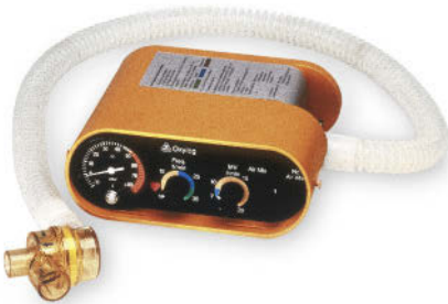
The first version of the Oxylog® ventilation device. Constant volume ventilation in emergency medicine
