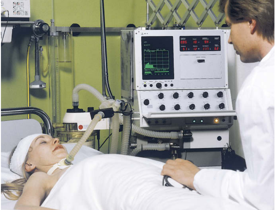
Intensive ventilation with EV-A. Depiction of the ventilation curves on the integrated screen
