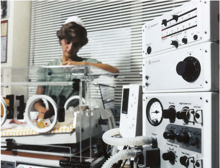
Babylog 1 for use in neonatal clinics. Additional modules connect to the ventilation device for setting the oxygen concentration and monitoring breathing pressure
