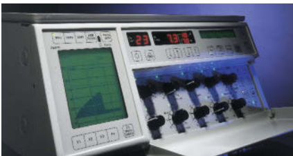
Monitoring devices on an Evita 2. The numerical values next to the graphics screen are ordered by priority
