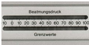
Airway pressure monitor on the UV-1 with depiction of limit values
