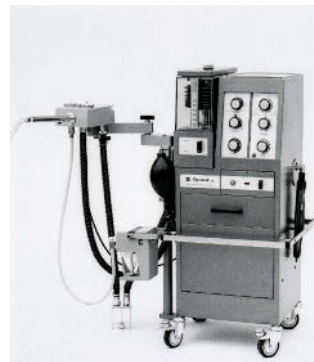
Spiromat 661 with ventilation head E for long-term ventilation of adults
