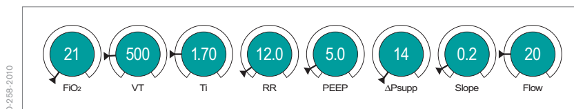
Figure 11: Possible ventilation settings
