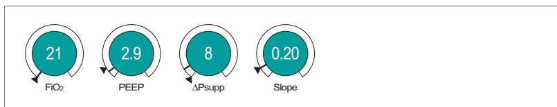
Figure 32: Possible ventilation settings
