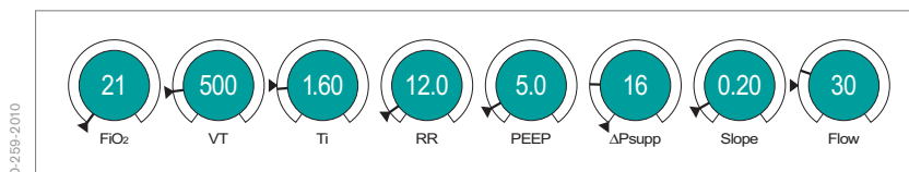
Figure 13: Possible ventilation settings
