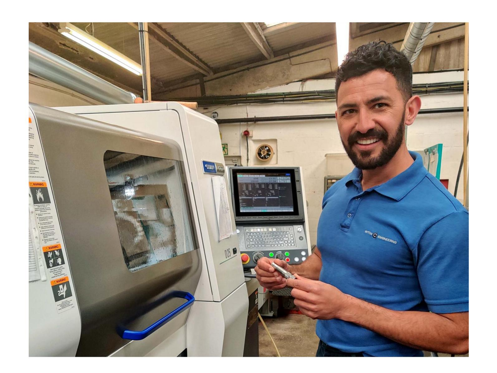
Witon Engineering's new 25mm bar capacity Citizen sliding head turning centre is taking work off bigger machines and cutting cycle times by 20%.
