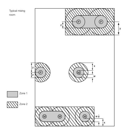
M = mixing vessel P = pump
