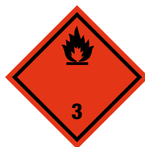
Figure 4 Labelling for Class 3
