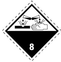
Figure 11 Labelling for Class 8
