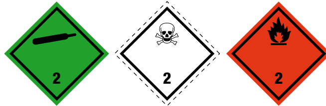
Figure 3 Labelling for Class 2
