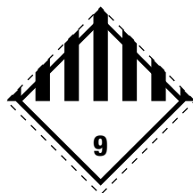
Figure 12 Labelling for Class 9
