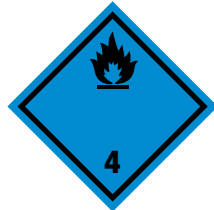
Figure 7 Labelling for Class 4.3
