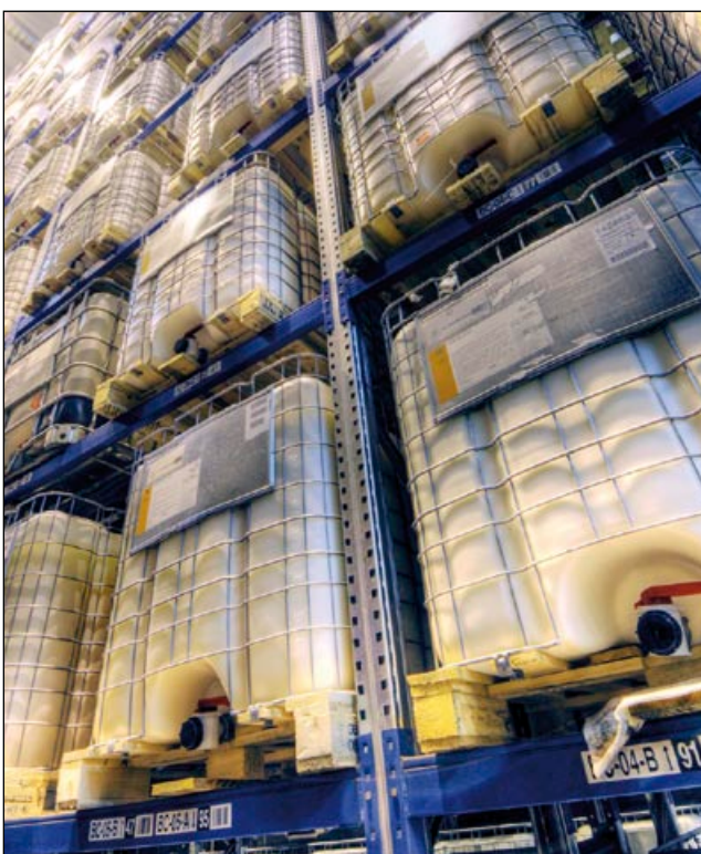
Figure 26 IBCs stored on warehouse racking
