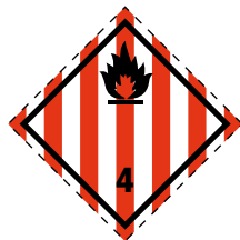
Figure 5 Labelling for Class 4.1
