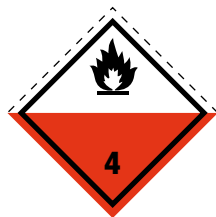
Figure 6 Labelling for Class 4.2
