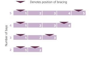
☐ This system does not need bracing if fully clad.
