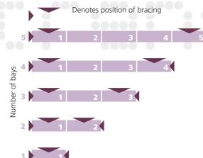
☐ This system does not need bracing if fully clad.
