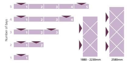
☐ This system does not need bracing if fully clad.
