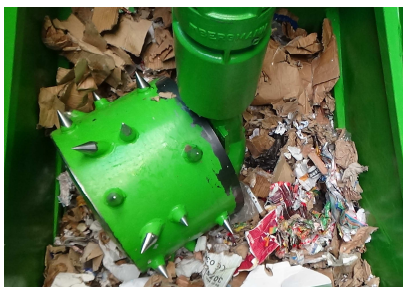
Functioning of the compaction-drum
