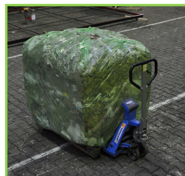
Bale of a Roto-Compactor PS 1400-E approx. 400kg
