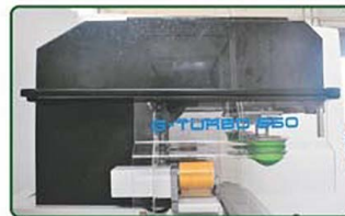
Stable granite stone machine structure
