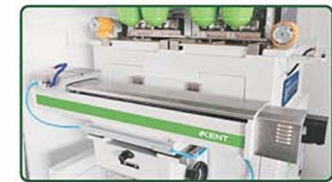
Precision servo product shuttle (DRE)
