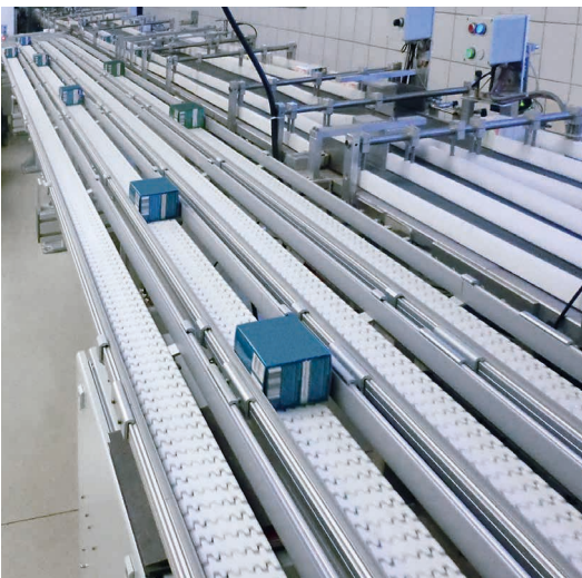
Versaflex flat top chain conveyor as a parallel multi-line system
