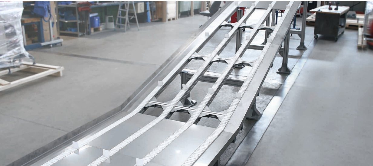
4-track Versaflex flat top chain conveyor A06 with cleats
