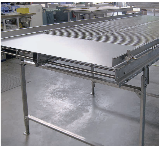
INOX gravity roller conveyor for transport of baked goods
