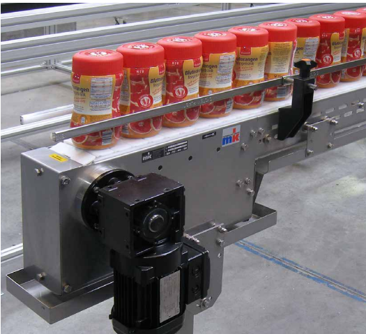
INOX flat top chain conveyor complete with drip pan
