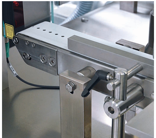
INOX vacuum belt conveyor with custom side rails
