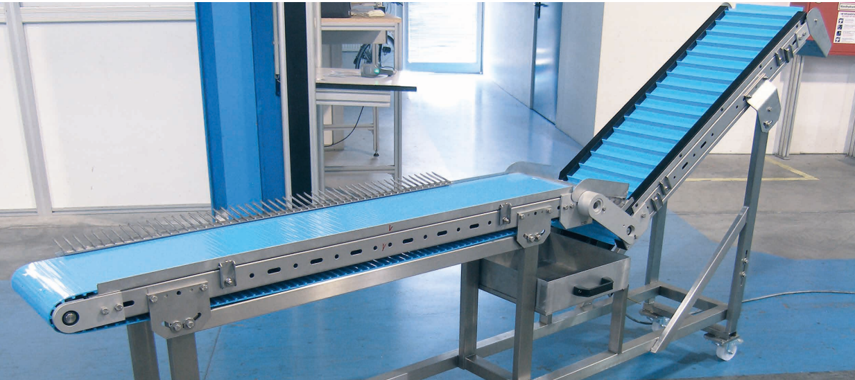
Combination of INOX belt conveyor and angled belt conveyor for transport of praline balls with granulate
