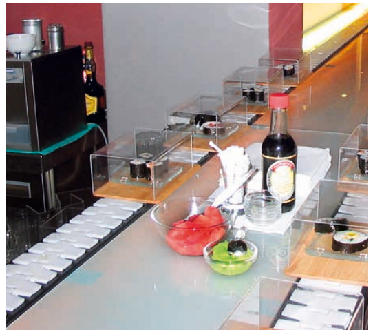
INOX flat top chain conveyor used in hospitality field
