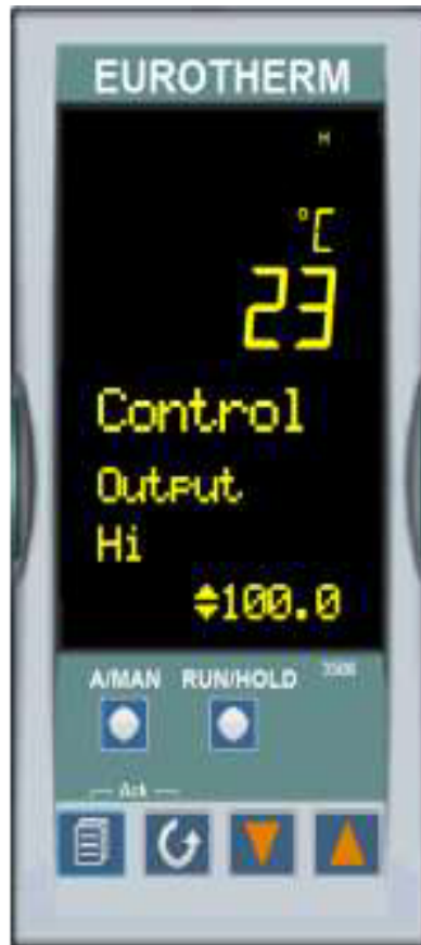
Power Limit View
