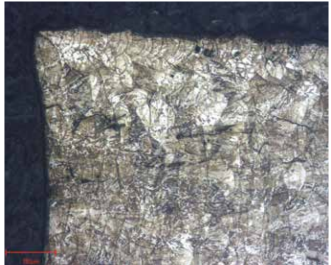
Fig. 7: Etched specimen using "V2A Beize" (for 45 s). Edge section. The microstructure is clearly discernible.
