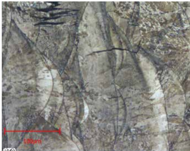
Fig. 8: Contrasted specimen. The welded-based microstructure of the manufactured workpiece is clearly visible.
