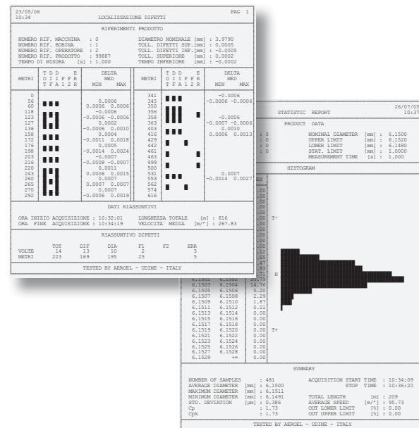
(\*) Only flaws which turn into a diameter change all along the product circumference, like "olives" or "neck-down", can be surely detected. The minimum detectable flaw length is given by the max line speed divided by the gauge scan frequency.
