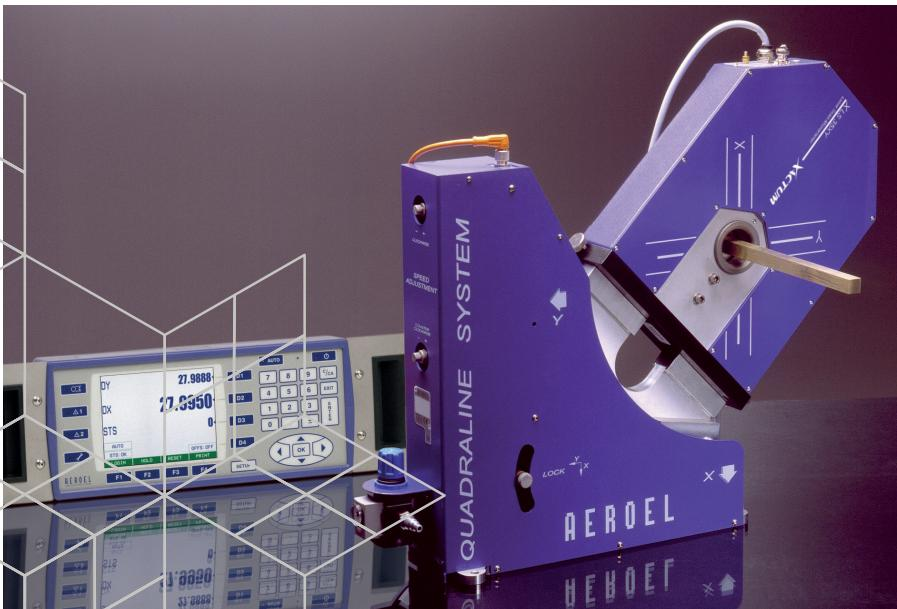
Quadraline.XY is a laser system designed to control the 2 dimensions, height (H) and width (W) of extruded or rolled products featuring rectangle-like cross section, such as metal straps, plastic or metal section, etc.
