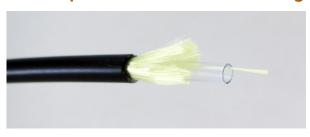
PVC over Kevlar over PTFE. Standard in the telecom industry because of the Kevlar members which prevent stretching. Ideal for small fiber sensors, D20 or RC20 and smaller. MRI compatible and liquid tight. Light crush resistance.
