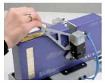
Selecting the **Auto-sync mode**, you will get one measurement only, triggered just after having positioned the sample and after a programmable delay. The display will maintain the measurement after you have removed the part.
