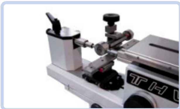
3) Checking of plain and threaded plug gauges using the floating table
