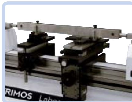
Checking of long series gauge blocks
