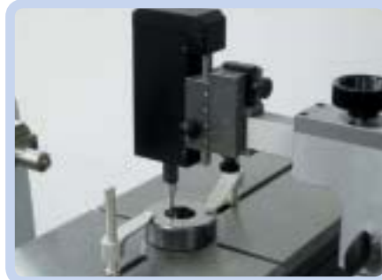
Plain ring gauge from 1mm up to 20mm
