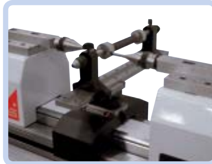
Checking of plug gauges
