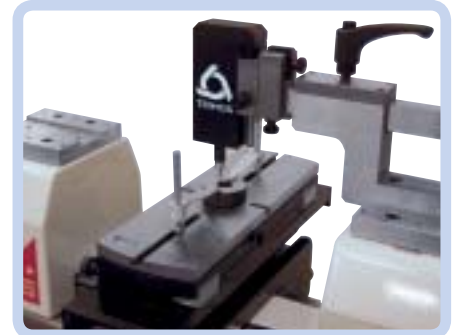
Checking of small ring gauges
