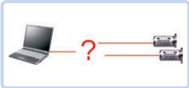
Standard configuration for ZEROTRONIC sensors. The customer can view and record the sensor output signal using their own in-house software.
