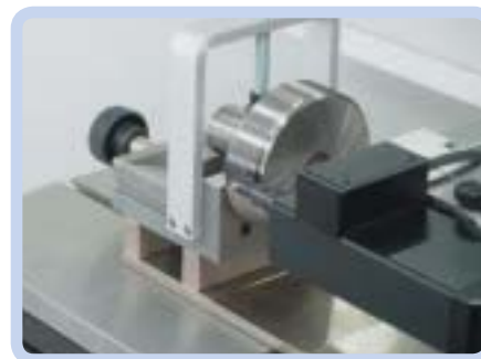
Checking of taper thread gauges (plug/ring gauges)
