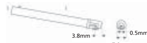
Transverse chisel probe for gauging sharp edges or small O.D., aligned to axis of traverse
