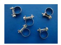
**Fuel hose clips, or Nut & Bolt type** clips offer the user a quick and safe way to attach a fuel hose in the vehicle. Simply fit the clip over the hose in the same way as a worm drive, and then tighten the screw. Because the clip has no housing attached under the band, just the 'Bridge' under the screw assembly, the band tightens almost 360° sealing. The look of the clip, when fitted, is simple and uncluttered. Very neat and tidy.
