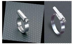
**FLEX GEAR** is the **MICRO GEARS** bigger brother. This design enables the user to clamp from 25 – 45 millimetres upto 210 – 232 millimetres. The **FLEX GEAR** uses precision manufactured spring washers under the head of the worm gear to ensure 'Cold Flow' is eliminated. The **FLEX GEAR** in built from wider band width stainless steel and uses either a 5/16<sup>th</sup> hex headed worm or for the 'Standard'
