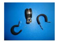
Rubber lined or plain '**P' clips** are found in all types of vehicles. The beauty of the clip is in it's simplicity to use. Snap the 'P' clip around the hose, bring the fixing holes together, apply the screw, job done.
