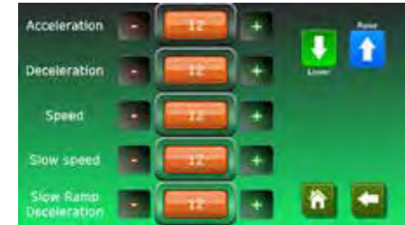
Gate and barrier speeds and slow down settings are on one page for simplicity.
