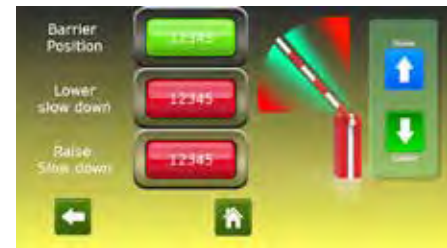
The gate or barrier can be operated from the screen to test the programmed settings.
