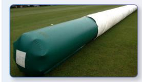
Used to roll covers out quickly. Made from PVC, the 3ft diameter tube is easy to manoeuvre. Inflated with an adapted leaf blower in as little as 2-3 minutes, depending on tube size. Flat sheets are attached to the cover using Velcro.
