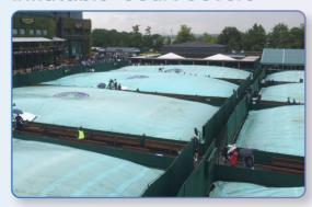
We produce the Inflatable Tennis Court Covers as used at the Wimbledon Tennis Championships. They are made from a lightweight material that, once rolled out across the court, are inflated by fans to form a dome allowing water to drain into channels around the court.
