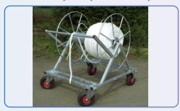
Heavy duty galvanised steel trolley with a central "bobbin" which holds two 220-metre boundary ropes. A handle winds the rope onto the bobbin. The Trolley features 2 swivel and 2 fixed wheels for easy manoeuvrability. Size: 1070mm wide x 1270mm long x 1350mm high.
