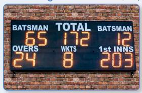
This fifteen digit scoreboard is designed to be a versatile scoreboard that can easily fit to the outside of a pavilion while being light enough to be removed. The scoreboard uses 250mm amber LED digits which create a bright and clear number. The Club Scoreboard displays both Batting Scores, Overs, Wickets, 1st Innings and the Total Score.
