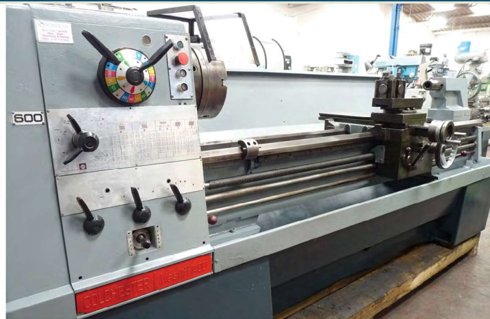
Colchester Mastiff 1400 80" Gap Bed Centre Lathe 80" (2000mm) Between Centres, 21" (535mm) Swing, 32" (815mm) in gap, 90mm bore
